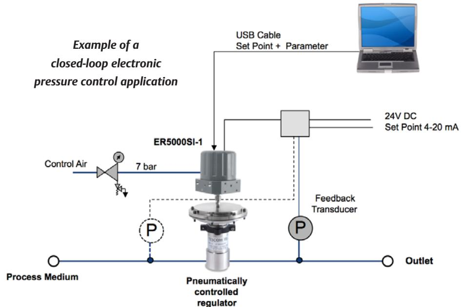
Electropneumatic PID controller with mechanical regulator produces output pressure equal to a command signal high ( $\pm 0.1\%$ ) accuracy when combined with an accurate pressure transmitter. (Photo courtesy of Emerson Process Management)
