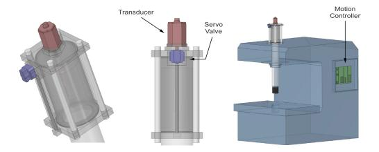
With the Moog servo valve applying the correct force, the Temposonics transducer precisely monitoring the speed, and the Delta Computer controller managing both control loops, the compacting press was able to perfectly execute its objective and outperformed the customer's specifications. Needless to say, the customer was thrilled.
